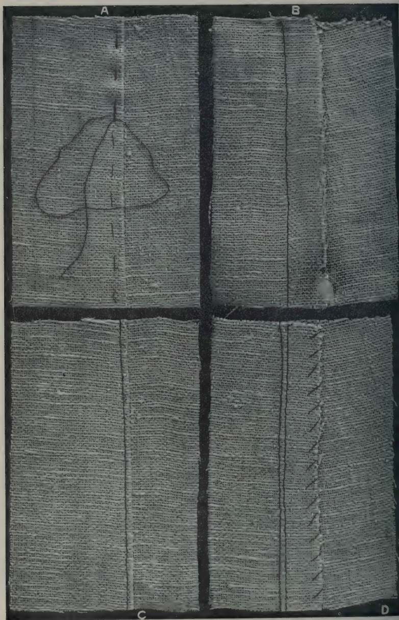
FIG. 199.—Cord seam; A , basting for outside stitching; B , wrong side before outside stitching; C , outside stitching; D , wrong side after stitching.
